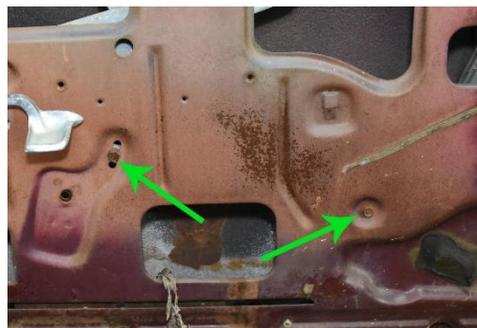
This image of the door glass, outside of the car, shows the 2 bolts for the rear window slide/stop and front window stop, identified with YELLOW arrows, that you are removing. Carefully roll the window up or down as necessary to get to each bolt.
