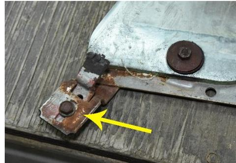
You will not need to remove the rear upper window stop to remove the glass from the door though you may choose to do so. If you do be sure to mark the bolt location prior to removing it to assist with reassembly.
